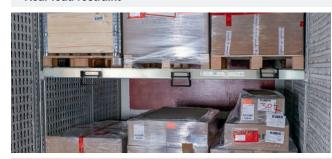
To secure the load to the rear, the last STD loading beam is secured with Pallet stops.
