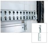
The KAT AJS 900 can be parked between the pillars, with the AJS holders, and the AJS lashing profile can be used without any restrictions. Due to the flat design of the AJS holders, the entire width of the vehicle remains unaffected. The AJS holders can be easily clamped onto the AJS lashing profiles. Tools are not required.
