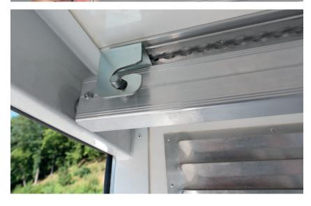
KIM locking bars are stowed securely under the roof for loading and unloading.
