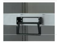
Before unloading, the Pallet stops are moved to the park position. In this position, the STD loading beams can be stowed under the roof.
