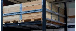
To achieve the maximum payload of the CTD-III decking beams, we recommend a grid size of 2,42 m for pillars. Consequently six euro pallets can be positioned in each stanchion area. CTD-III decking beams which are not in use can be parked between the pillars. Larger pillars intervals enable loading from the rear and the side.
