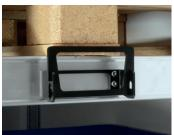
Three Pallet stops are attached to the last STD loading beam. Once the STD loading beams have been loaded, the Pallet stops are manoeuvred easily into the restraint position.
