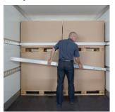
simply unlock the locking deviceon one side.
