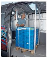
and to comply with weight distribution regulations, cargo should be loaded towards the back and in the middle of the floor surface.
